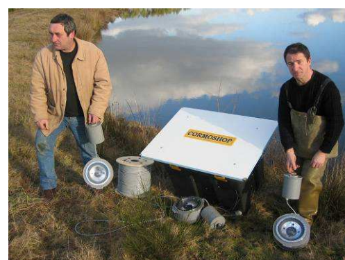
Even installations that produce the sounds of orca whales are used to scare away cormorants temporarily.
